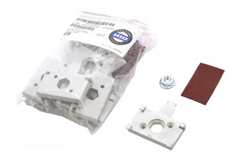
The Omnikey Contactless Reader Mounting Bracket is designed to offer an easy way of mounting certain Omnikey readers. The bracket comes complete with a standard photographic screw nut and countersunk screw holes, enabling the reader to be screwed to various surfaces and tripods, plus a matching self-adhesive pad, offering an alternative option to secure the reader without screws.
